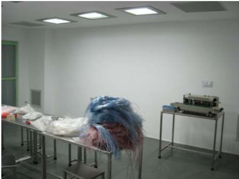
Medical devices assembled in class 10,000 Clean Room
